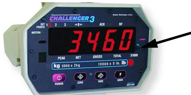
Figure 5-1. Calibration Button Seal Screw
