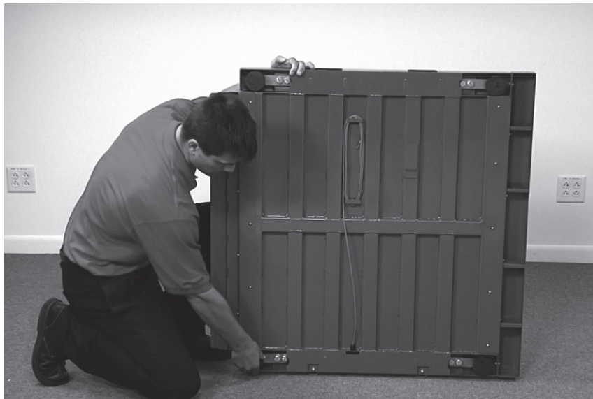
Figure 3-3. Backing Out the Scale Feet
