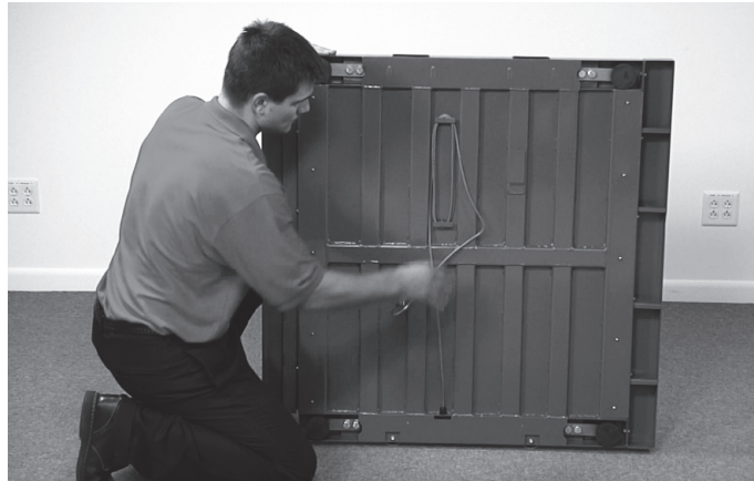
Figure 3-4. Unwrap the Cable from the Underside of the Scale
