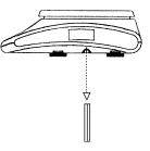
• If the scale will be stored or transported in the future, save the packaging material and re-install the protection screw to ensure the best possible protection for the scale.
