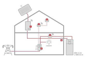
A full Energy Management System implementation provides the best holistic solution for connecting the STIEBEL ELTRON WWK hot water heat pump to a solar PV system. The EMS will activate the WWK to heat water at the best possible time to reduce consumption from the grid.
