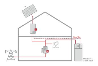
SG Ready implementation of connecting the STIEBEL ELTRON WWK hot water heat pump allows for a higher water temperature and more "free" hot water. A signal wire is connected from the solar PV inverter \* to the WWK, activating a higher secondary water temperature set point.
