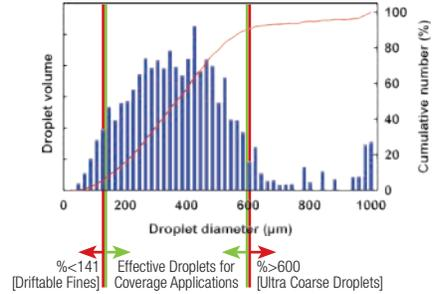
SR series droplet distribution balances excellent fine spray coverage while reducing driftable fines.
