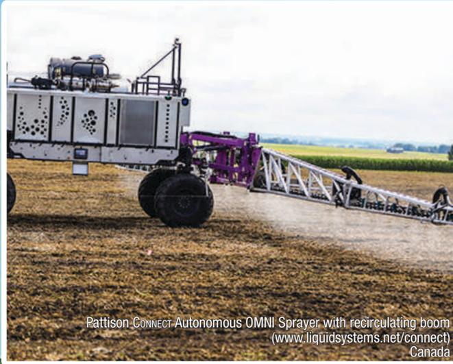
Pattison CONNECT Autonomous OMNI Sprayer with recirculating boom
