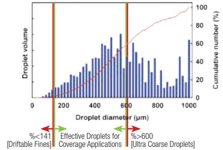
DR series is designed to produce extremely coarse spray with very minimal drift.
