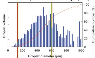
MR series is designed to produce relatively coarse spray with minimal drift.
