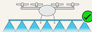
UAV sprayer applicators are able to use DX nozzles for targeted spray applications, but often due to boom constraints or UAV sprayer outfitting, wider angle nozzles like the MR110° nozzles might be used. In specialty circumstances that require a narrow full pattern spray can take advantage of the DX series of narrow-angle nozzles.
