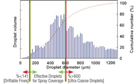
UR series is designed to produce ultra coarse spray with extremely little drift.
