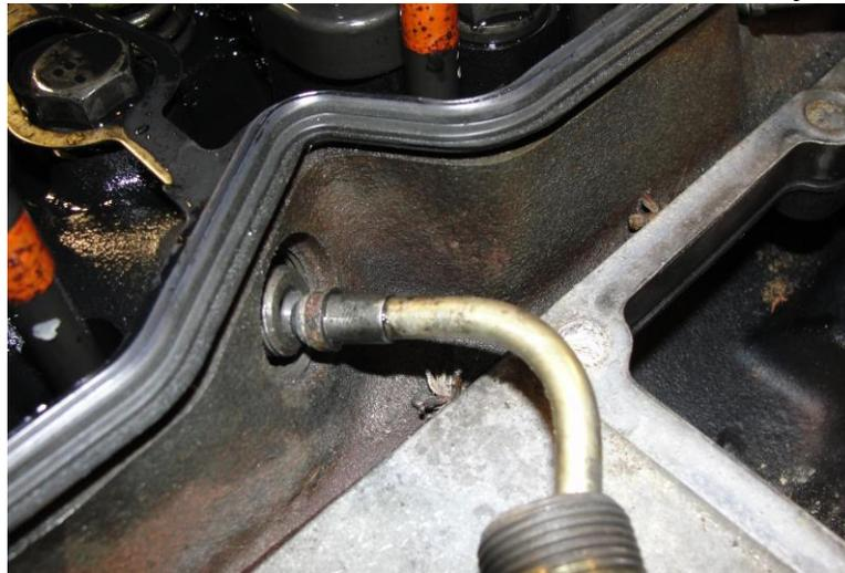
8. Remove valve cover. Pushing down on the leader hose, slide valve cover up and left.
