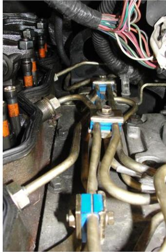
6. Remove rear engine lifting bracket (15mm socket)
