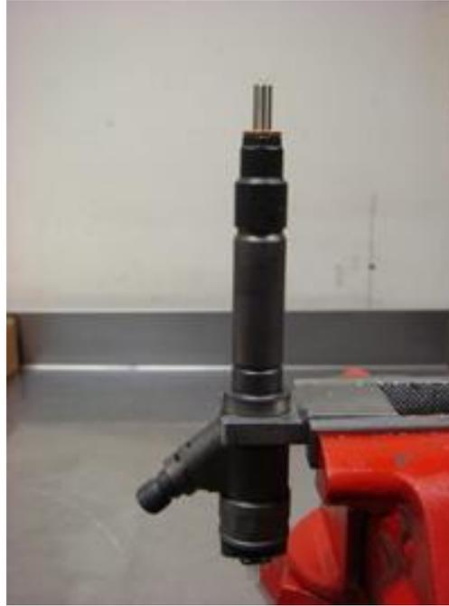
4. Using pliers, remove the copper sealing washer. If you are missing the copper washer be sure to dig it out of the cylinder head before putting the injectors back in. Some carbon buildup may be present and this is normal. Sometimes the carbon may seem excessive but there is no reason to worry. Do not clean the nozzles for us. We use an ultrasonic machine to gently clean the nozzles without damaging them.
