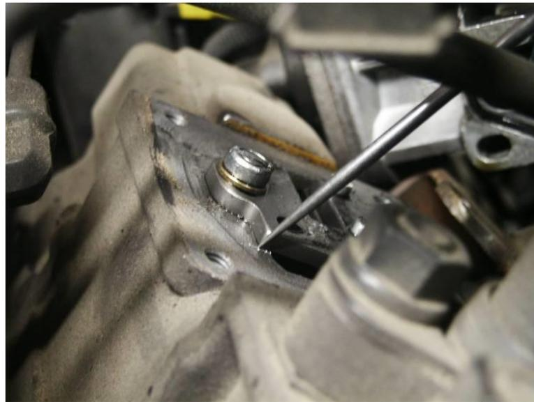
14. With a flat blade screwdriver, remove the stock fuel plate.
