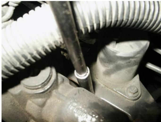
10. Rotate fuel shutoff solenoid out of the way toward the driver's side fender.
