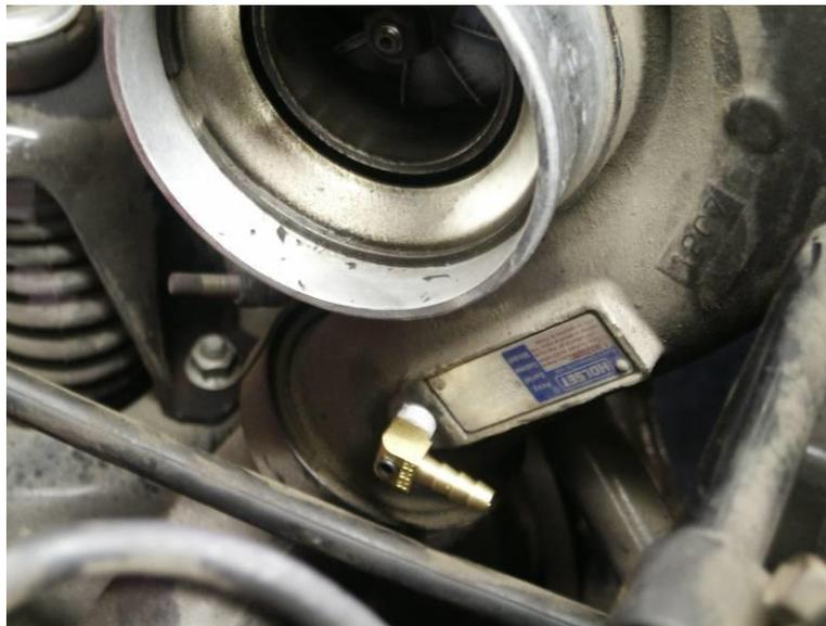
26. Reinstall boost reference line with the new supplied hose clamp.
