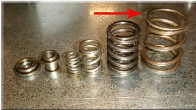
13. Use caution when installing the new DDP seat and springs (be especially careful to ensure you **DO NOT** drop any parts into the injection pump). Reinstall the DDP springs in exactly the same location they were in when you removed them. Preload the springs to the same amount of clicks you counted upon removing the old springs. Typically this will be 2 or 3 clicks. If need be you can also reference the measurement you took prior to fully removing the factory springs.
