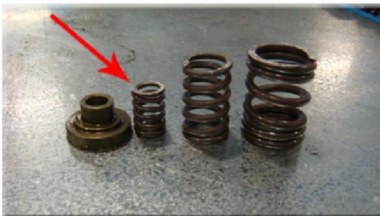
This photo displays 3 governor springs. The *smallest* spring (indicated by the red arrow above) should **NOT** be used with the 160hp, 175hp or 180hp pumps. *Without* the small spring installed, you should expect 3,000 - 3,200 rpm engine free rev. *With* the small spring installed, expect about 4,000 rpm engine free rev.
