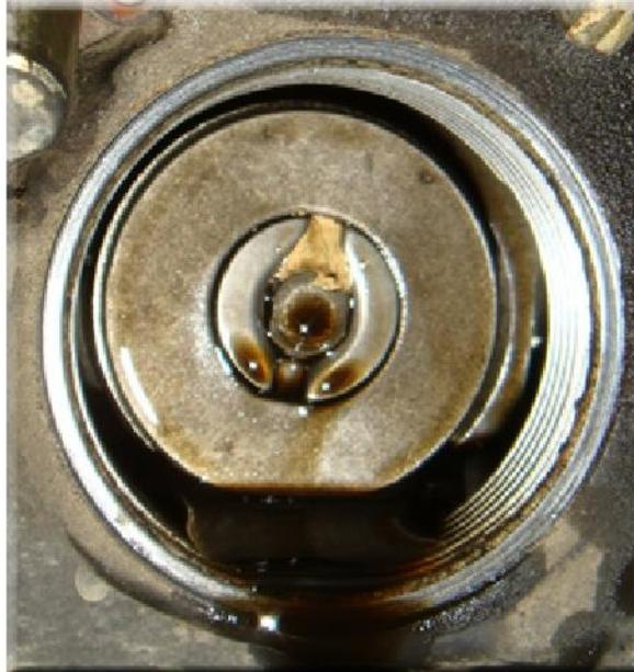
10. Using vernier calipers, measure the depth from the top of the stud to the bottom of the groove. Note this measurement as you may use it during reassembly. Every 90 degrees, you should count 1 click.
