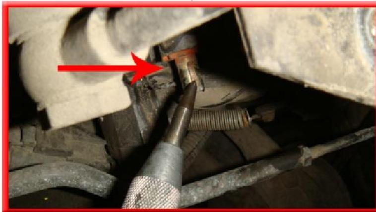
6. Once the fuel shutoff arm is out of the way, there is a wire that must be broken to access the 7/8" plug (located under where the fuel shutoff solenoid was). This wire can simply be broken with pliers.
