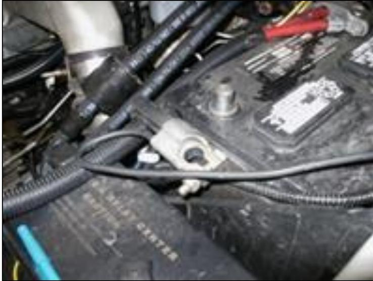
2. Remove 10mm bolts that hold intake, dipstick, and wiring.
