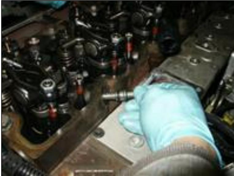
32. Replace connector tube nuts and finger tighten.
