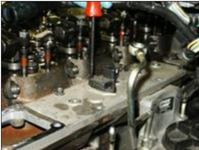
19. Remove 15mm rear engine lift bracket bolts and bracket.
