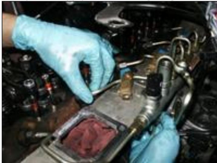
39. Connect high pressure supply line, and finger tighten.
