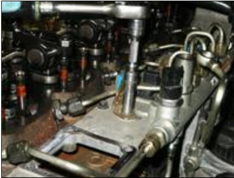
16. Remove 10mm bolts holding fuel rail.
