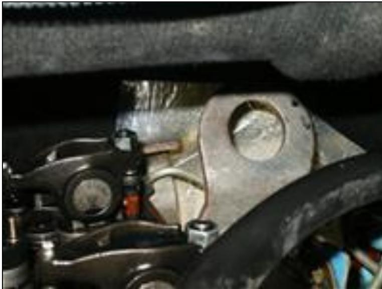
14. Remove 13mm bolt from rear fuel line holder. (04.5 and up only)
