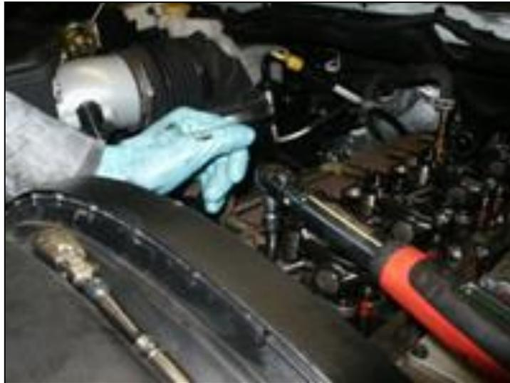
36. Reinstall engine lift bracket torque to 57ft lbs.
