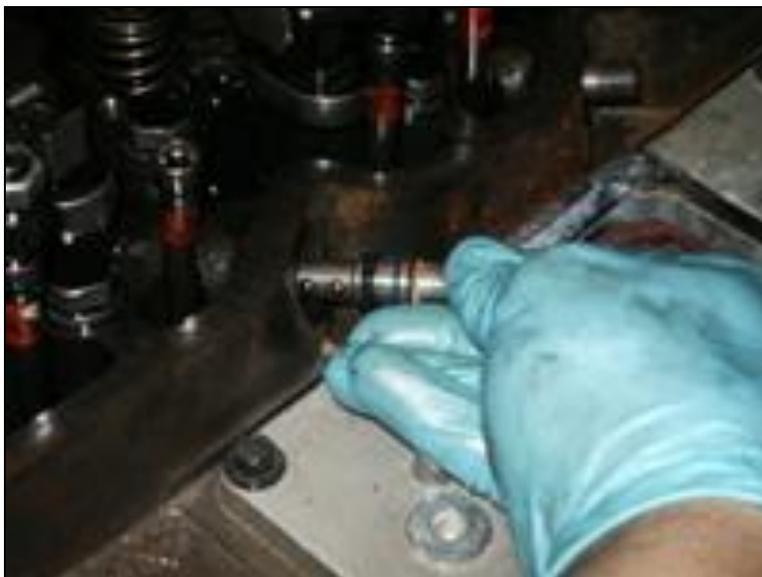
22. Remove 8mm injector hold down bolts.
