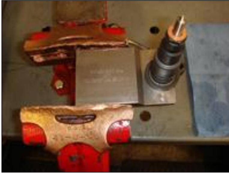
25. Remove Copper washer from old injector nozzle with pliers taking care not to damage the nozzle.
