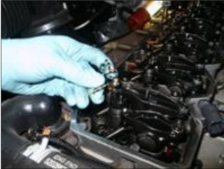
7. Remove 10mm bolts holding riser box.
