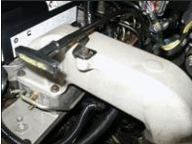
3. Remove 11mm Intercooler boot clamp.
