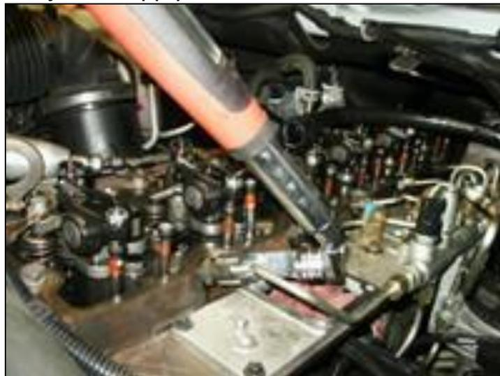
42. Install fuel line hold down bracket at rear of fuel rail, and torque to 18ft lbs.
