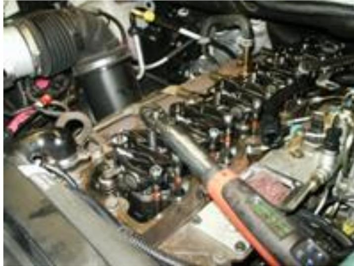
48. Install riser box, and torque to 18ft lbs.
