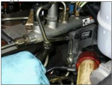
11. Disconnect fuel return line from pressure limiting valve, and bend gently out of the way.
