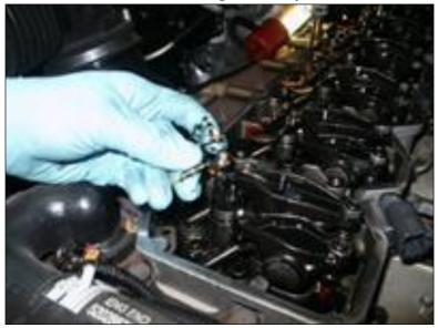
7. Remove 10mm bolts holding riser box.
