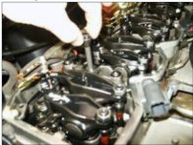
8. Remove 10mm bolts holding exhaust rocker arms, these are in the middle of the rocker, and sometimes covered in oil. Make sure to keep track of which cylinder these came from.
