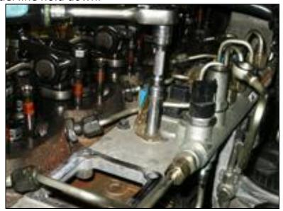
16. Remove 10mm bolts holding fuel rail.
