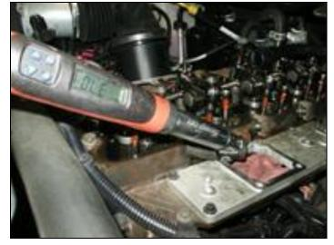
35. Torque injector hold down nuts to 89in. lbs.
