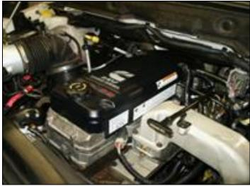
56. Reconnect negative battery cables, and start truck. There will be some smoke at startup that should go away within 30 seconds or so. If the truck does not start check connector tube torque. Under no circumstances should the high-pressure fuel lines be loosened to bleed.
