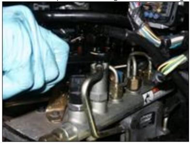
12. Disconnect 19mm high pressure lines from injector connector tubes.
