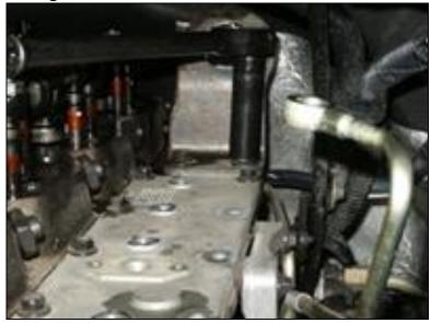
20. Remove 24mm nuts holding high pressure connector tubes.
