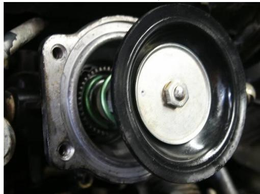
11. Reinstall the AFC cover, and the TPS if equipped.
