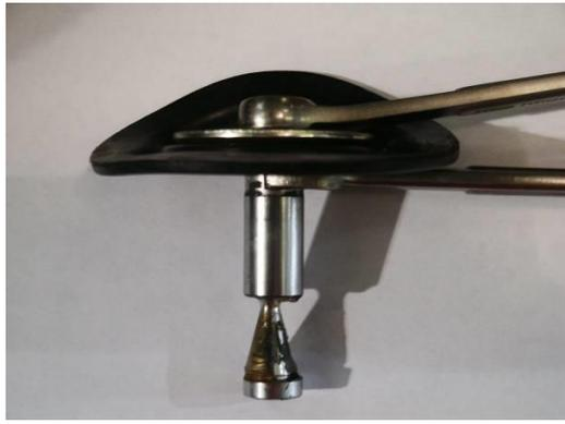
7. Install the diaphragm and washers on the new Power Pin. Be sure to locate the punch mark on the top washer so that it is exactly in line with the face of the cut on the pin.
