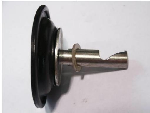
9. Lubricate the Power Pin.
