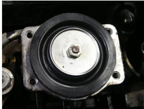
4. Remove diaphragm by gently turning and lifting.
