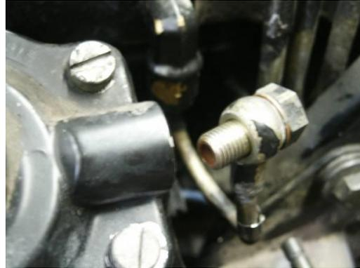
3. Remove the 4 cap screw on top of the AFC cover, and remove cover.
