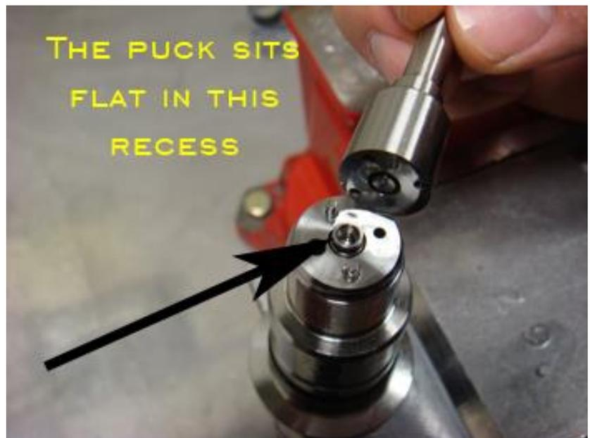
\*Note: For 5.9 injectors, there are two different style pucks that were in these units. Our nozzles will work with both designs shown here, simply follow the same install procedures.
