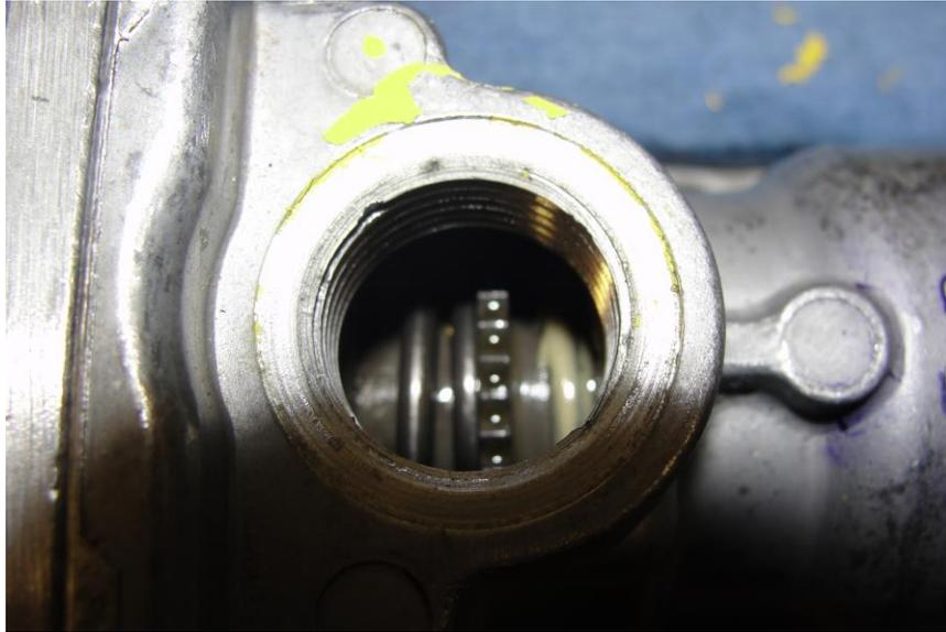
11. Adjust Star Wheel until it is in the center of the window for initial testing.
