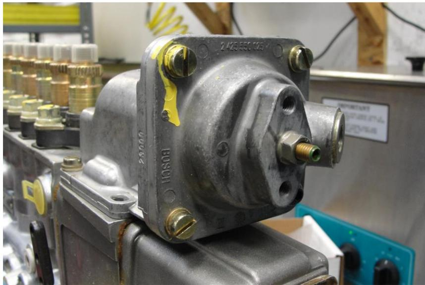
5. Remove rubber diaphragm. (This is spring loaded, so be careful. Take note on how the fender washers are installed.)
