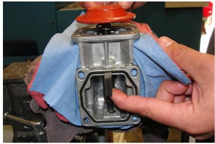
8. When installing the rubber diaphragm, make sure the radius of the fender washers are AWAY from the rubber. This insures that the diaphragm will not get cut
