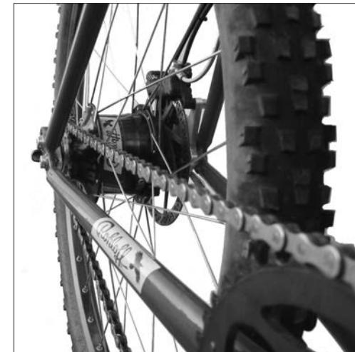
Rohloff SPEEDHUB 500/14 CC DB OEM mounted in a frame with adjustable Rohloff OEM dropouts
