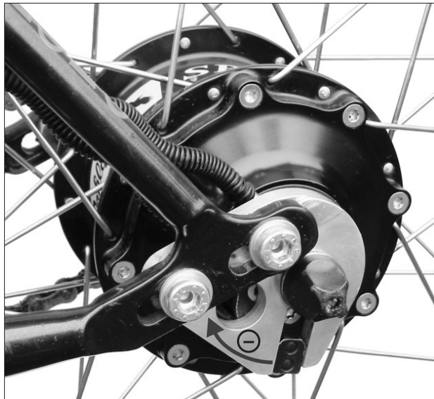
Rohloff SPEEDHUB 500/14 CC OEM mounted in a frame with adjustable Rohloff OEM dropouts
