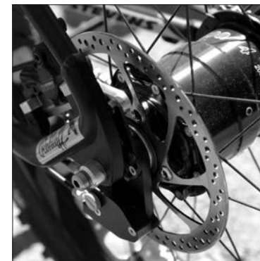
Rohloff SPEEDHUB 500/14 XXL A12 DB OEM2 mounted with the Rohloff FAT BONE and a disc brake
