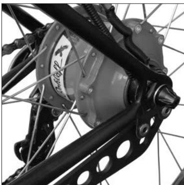
Rohloff SPEEDHUB 500/14 CC mounted with a long torque arm
