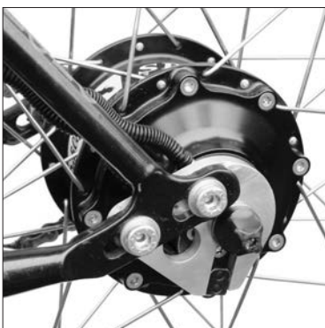
Rohloff SPEEDHUB 500/14 CC OEM mounted in a frame with adjustable Rohloff OEM dropouts
