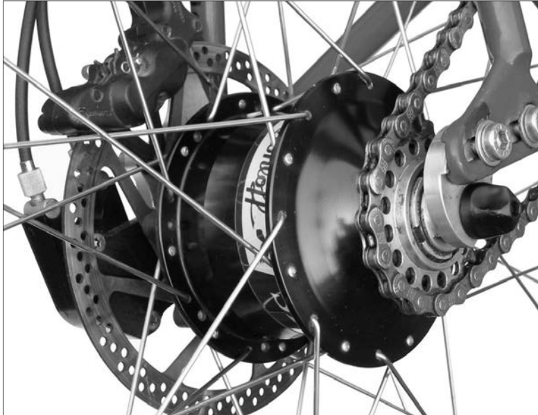
Rohloff SPEEDHUB 500/14 CC DB OEM mounted in a frame with adjustable Rohloff OEM dropouts
