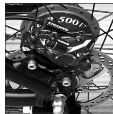
Rohloff SPEEDHUB 500/14 TS DB OEM2 mounted with the Rohloff MONKEY BONE (IS-PM Adapter) and a IS 2000 disc brake
