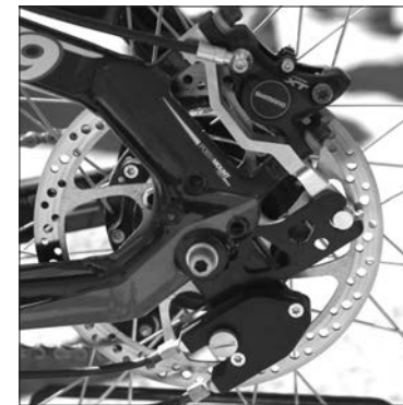
Rohloff SPEEDHUB 500/14 A12 DB PM mounted with the Rohloff PM BONE (PM-PM Adapter) and a PM disc brake
