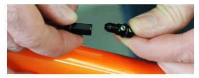
Use your cable splitters to separate the gear box cables and rear brake cable. <u>Note</u>: turn only the female side of the splitter (side with no set screws) counter clockwise to remove.
