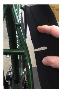
Note: When notching the frame padding, only cut half-way across the width of the padding. Also, the height of the cut or notch should match or be slightly less than the height of the obstacle. In this example we're cutting around the seat-stay bridge. The same process would be used for a brake mount.
