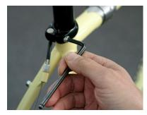
Use an Allen wrench to loosen the seat post clamp and remove the seat post with saddle attached. Turn the bolt counterclockwise to loosen but do not remove the bolt. After the post has been removed re-tighten the bolt slightly so it won't come out during transit.
