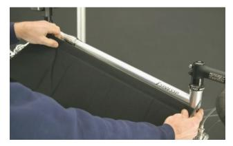
Take the next widest (3.75") roll of padding and measure correct lengths needed for the chain-stay tubes and fork legs. It may be necessary to notch the padding on one section to clear the disc brake tab on the fork. The remaining 2.25" wide padding will cover the seat-stay tubes.
