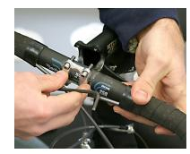
Use the appropriate Allen wrench to remove the handlebar stem's faceplate. Replace the faceplate and bolts after removal so that the parts don't get lost.
