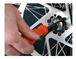
Now you can remove the wheels and fenders if installed on the frame and fork. We recommend removing the disc brake rotors from the hubs to ensure they stay true during travel. You will need either a Torx T25 wrench or a Centerlock tool depending on your rotor type.
