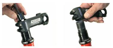
Next remove the stem's top cap, typically with a 5mm Allen. Loosen the stem's pinch bolts with an Allen wrench and remove the stem. Take careful notes of the orientation of spacers and headset parts. You will need this for installation later.
