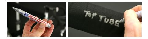
It is helpful to mark the padding sections with a paint pen or silver permanent marker (available at home improvement or craft stores). This will help for future identification and placement. With the fork removed and all accessories aside, we can now separate the frame into two sections by fully loosening each frame coupler. Turn toward the non-drive side of bike.
