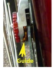
Road-type **caliper brakes** have a simple quick release which should be opened before removing the wheel.
