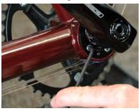
side, requiring a 4mm Allen wrench. We recommend a ball -end Allen tool such as those made by Bondhus to ease access to the screws. Back each
