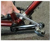
Most pedals can be removed with an a 15mm open-end wrench or 8mm Allen. Keep the right tool in your kit! Note: the left pedal is reverse threaded. Turn clockwise to remove. Upon reassembly, avoid overtightening to ease removal next time you travel.
