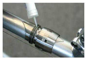
The S + S couplers on your Co-Pilot have been lubricated here at the factory. That lubrication is typically adequate for three years. S + S Machine recommends high Tefloncontent grease for continued trouble-free operation.
