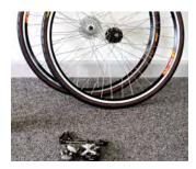
Now undo the wheel quick releases and remove the wheels. Remove the QR skewers from the axles and place them with your other parts.
