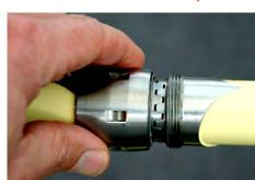
Now is the time to fully loosen each coupler and separate the frame sections. Make sure that all frame padding is securely fastened.
