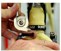
For **linear-pull** brakes, grasp the front brake so that the pads are pushed against the rim and remove the travel agent or cable guide from the right brake arm.
