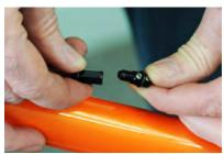
Grasp each end of your cable separators and turn counterclockwise (they should be just finger-tight) to release the cables for the rear brake and both derailleurs.
