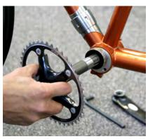
Pull the left arm and spindle out of the frame and bottom bracket assembly. Keep an eye on small washers and spacers, which will have to be reinstalled just as they were.
