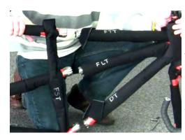
Keep cables out from under the padding. Pull the padding over the exposed coupler ends and Install the remaining padding.
