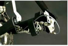
Pull the rear derailleur cage forward and strap it to the chainstay with two narrow strips of your frame tube covers.
