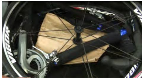
Now place the front wheel atop the rear wheel and rear section. Here you can see some heavy brown paper has been used to cover the cogs and keep the axles from banging together.
