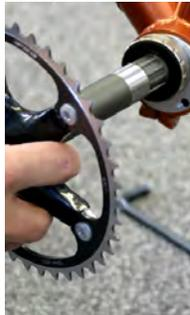
counterclockwise, you will encounter resistance, but **keep going**. Slide the spindle out of the bearing assembly after the free arm is removed.
