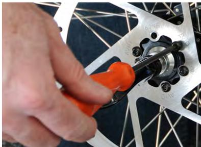
If you have discs, we recommend removing the disc rotors to ensure that they stay true. A padded mailing envelope is a great place to stow them in the case. The bolts can be threaded back in to prevent loss while traveling.
