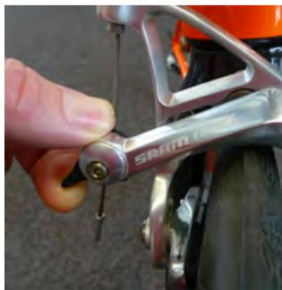
Before removing your wheels, open the brake caliper quick releases so that your tire doesn't hang up on the brake shoes. You may have to deflate the tires somewhat if you have larger tires.
