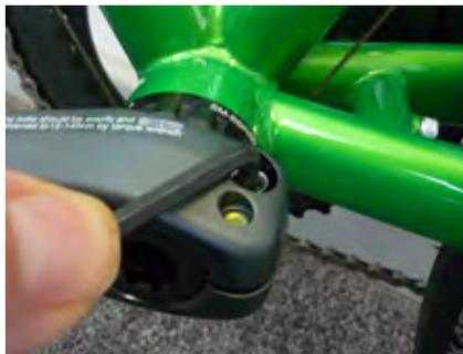
The second most-common system facilitates crank removal with two simple binder bolts, as shown. Loosen the bolts with an Allen wrench and the crankarm will come off. Slide the spindle out of the bearing assembly after the free arm is removed.
