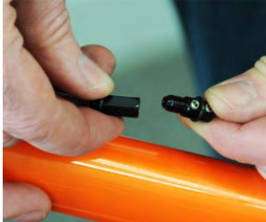
Grasp each end of your cable separators and turn counterclockwise (they should be just fingertight) to release the cables for the rear brake and both derailleurs. We will let the cables hang for now. After the frame is fully padded, we will coil up each cable to prevent tangles inside the case.
