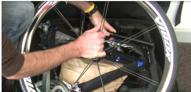
Do a final check to make sure that all painted surfaces are protected. Stuff rags or wadded paper into corners and over any parts that appear unprotected. Make sure there are **no loose parts** that might rattle around inside the case!
