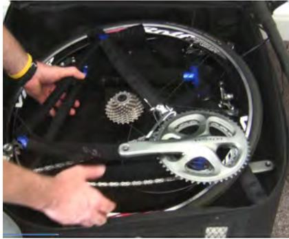
Work the rear frame section into place, passing the left crank arm between the spokes and under the rim, resting on the bottom of the case and pointed toward the corner of the case. The rear drop-out section should be on the opposite side of the case from the head tube.
