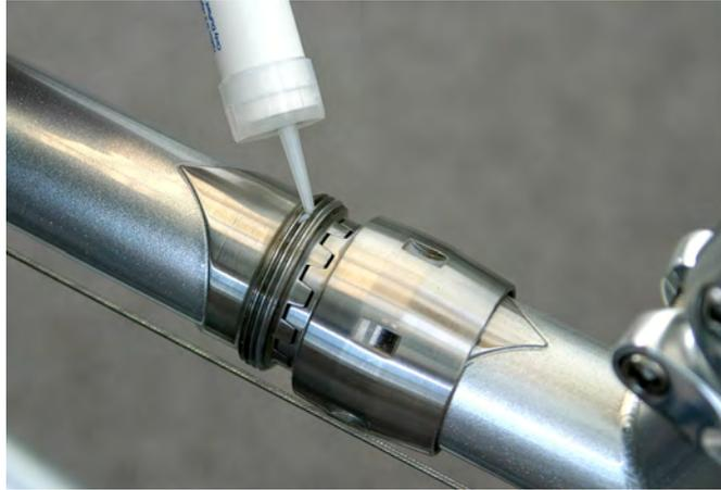
The S&S couplings on your Co-Pilot have been lubricated here at the factory. That lubrication is typically adequate for three years. We recommend high-Teflon-content grease for continued trouble-free operation.
