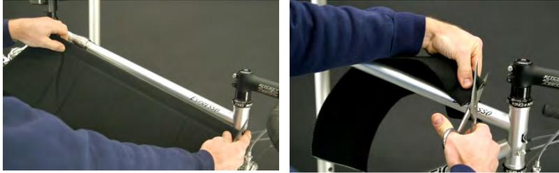
Notches may be cut in the padding where components are mounted. Hold the padding against your frame to find where notches must be cut.
