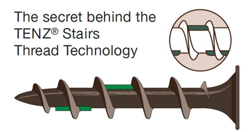
The stairs called "Stairs of the Peak (SP)" and "Stairs of the Vale (SV)" are located along the thread and their precise shape makes it possible to displace the wood fibres in a gentle way. The interplay between the pair of stairs makes the TENZ® Stairs Thread Technology so unique.
