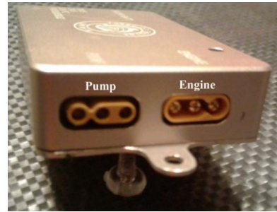
Figure 8 Pump and Engine Connection
