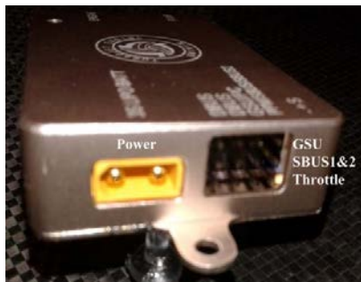
Figure 9 Power ECU Connections
