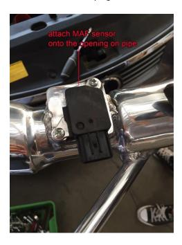
Now install the air filter and install the intake system as picture below. Use provided M8 absorber install below where the metal mounting bracket is located.
