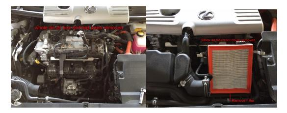
Once the top part of the air box and filter are removed, remove the 10mm bolt and bottom of the air box should come out. Note: some wire clips may be attached to the air box and please use a small flat head screw driver to unclip it from the air box. Next, remove the last 10mm bolt that is holding the intake tube.
