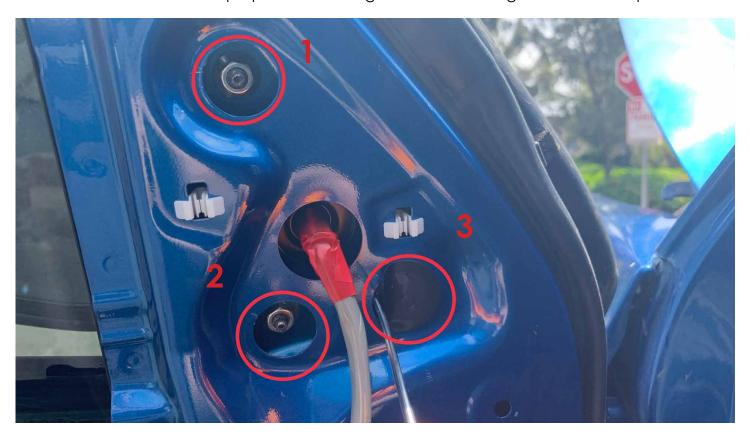
**2-C.** Remove three nuts off the mirror bolts passing through the door with a 10mm socket while holding the mirror on the outside of the door so it doesn't fall
