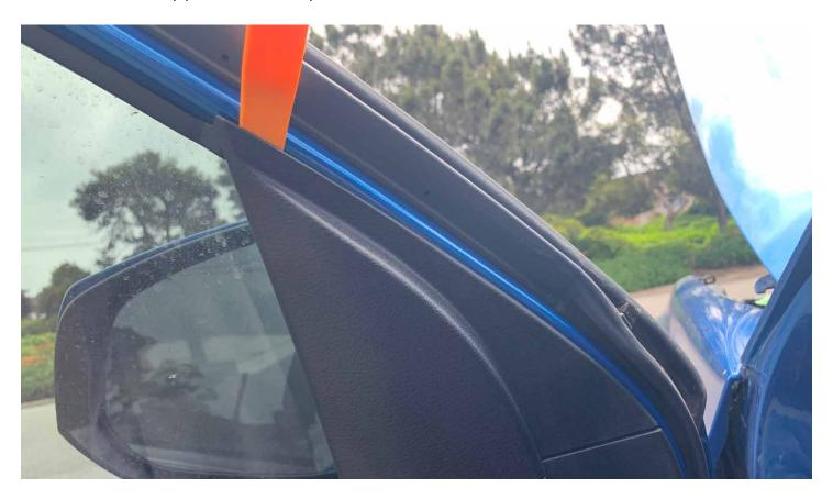
**1-G.** Remove door panel with trim removal tool starting at the bottom pulling hard and sliding up towards the window
