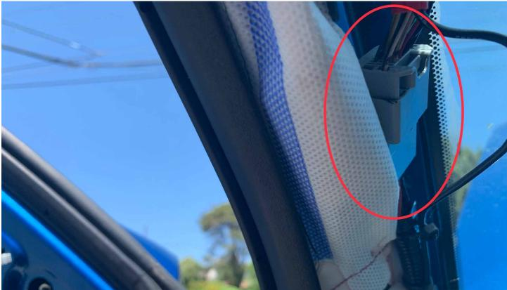
**4-G.** Tuck the extra slack of the meso harness in ensuring nothing is getting in the way or possibly interfering with the airbag
