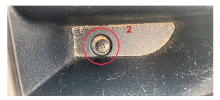
1-E. Push the center button in, located on the plastic panel and then pry outside with pick
