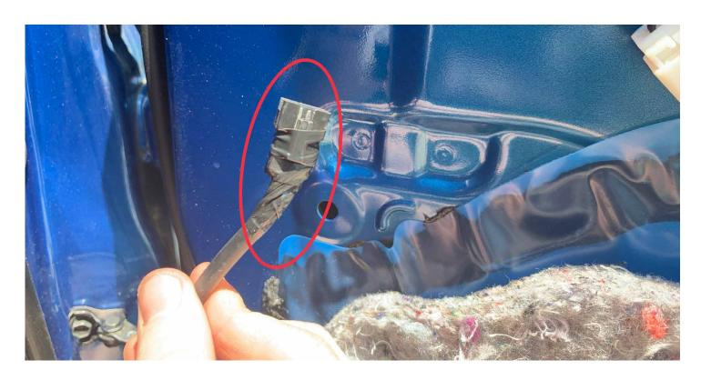
3-1. Feed the meso cable through the cab pass through to outside
