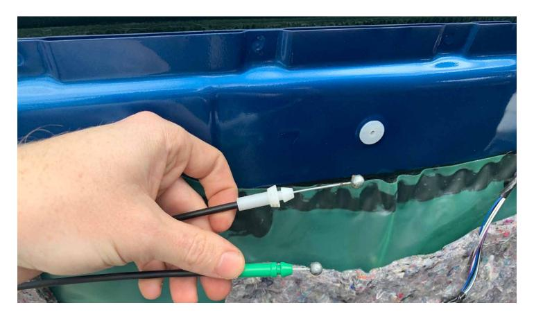
**1-I.** Disconnect the first of two electrical plugs, the larger plug has a release tab you press down and a collar that slides back.
