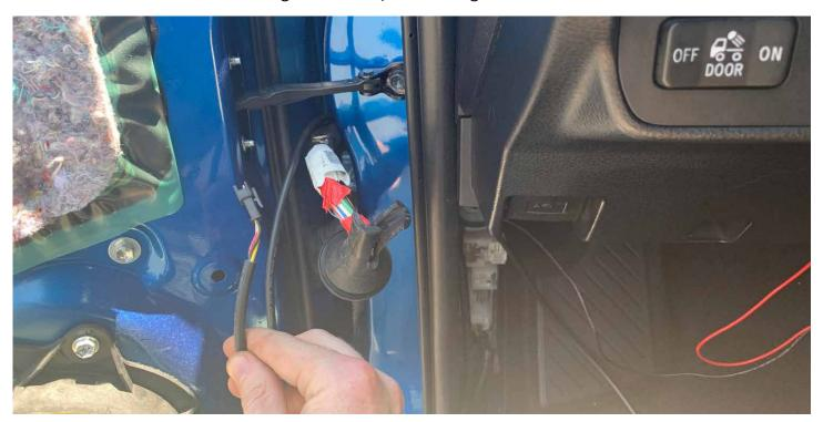
**3-J.** Push the connect through the boot which is a little bit of a pain in the butt but have patience, it helps to have one hand stretch the boot as you use the other hand to push the connector through with your finger, once you get it more than halfway you can roll the opposite side of the boot back to expose the connector and pull it the rest of the way, be very careful to not rip any of the factory cords or damage the boot
