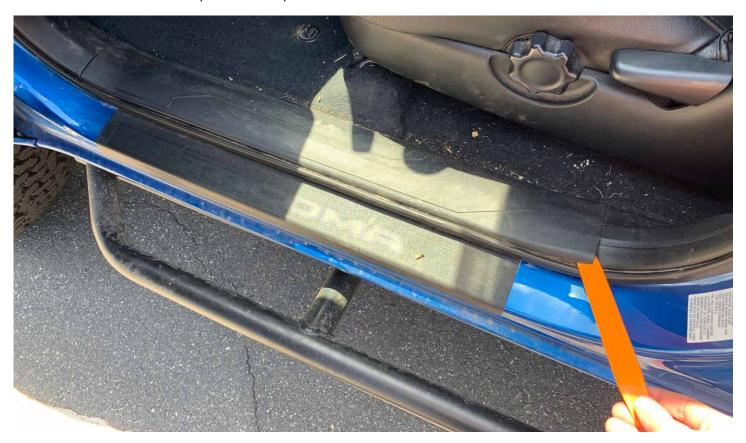
3-D. Remove twist cap nut with your hand and then pull side foot well panel trim piece out
