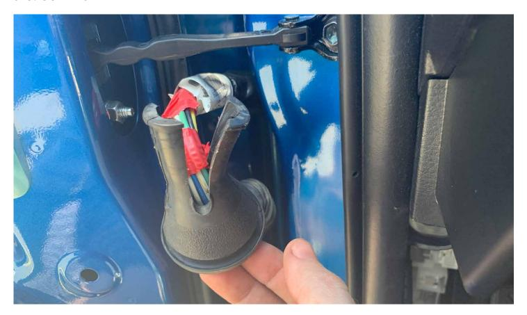
**3-H.** Take the shorter lead side of the meso harness and add some tape around the extension connector and its wires (if required) so the wires don't pull out and so the connector release tab doesn't snag on the boot as you push it through
