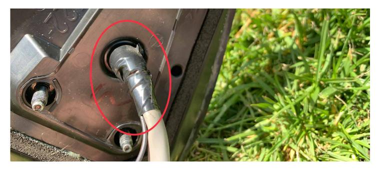
**2-M.** Reinstall mirror from outside door with 10mm socket to reinstall the nuts onto the bolts while passing the cords through the door and holding the mirror in place
