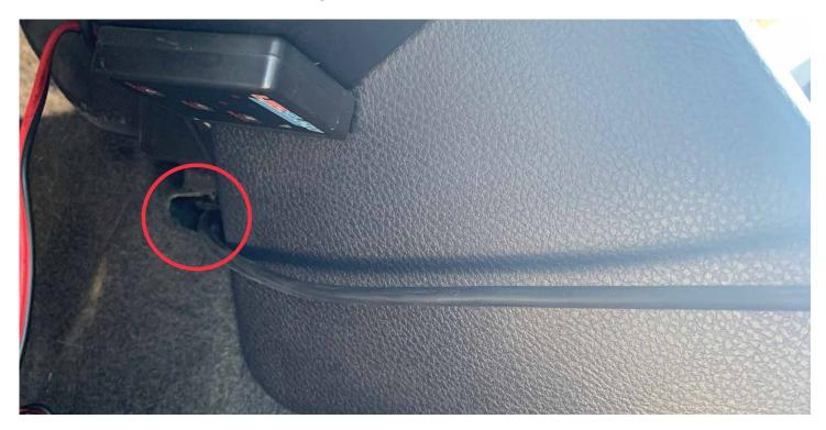
3-N. Feed cable under carpet in passenger foot well, it just lifts up
