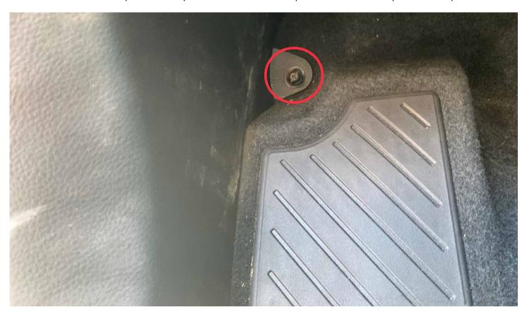
3-E. Disconnect three plugs in the driver foot well
