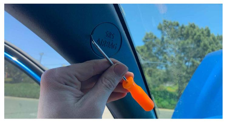
4-D. Use the 10mm socket to remove the bolt and pull the a pillar cover off
