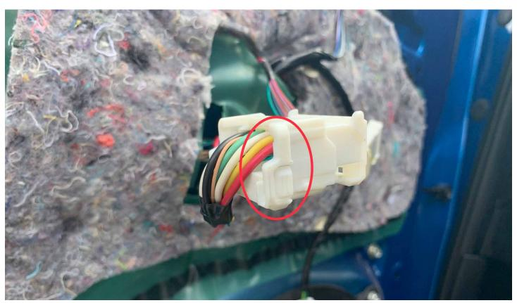
**1-J.** Disconnect the second of two electrical plugs. The smaller one has a release tab you press down.
