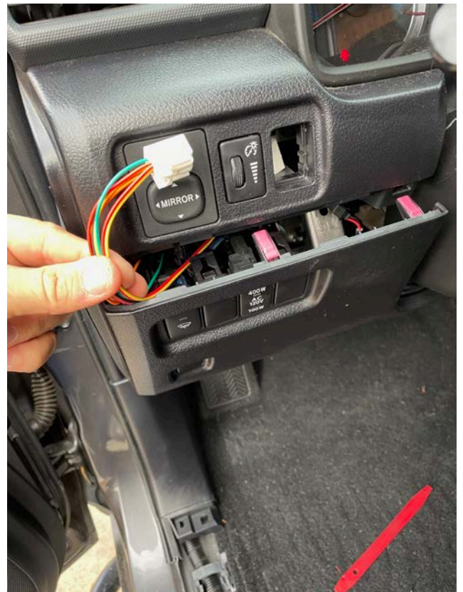
STEP 8: ROUTE MAIN PLUG UP BEHIND DASH
