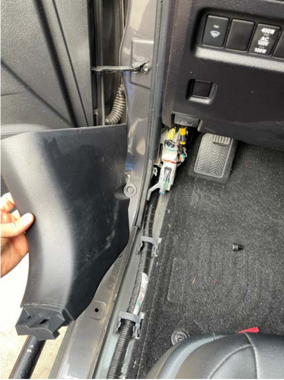
STEP 1: REMOVE DRIVERS KICK PANEL
