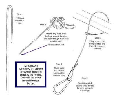
Stretch the net out on the ground and loosely tie off each corner to the vertical poles and raise the net up as high as you can. You will probably get it about 6' high. Connect some of the hangers to the top of the net near the center of the frame. Raise the corners up more, and keep adding hangers going toward the ends of the frame. Once all of the hangers are in place, tie the corner ropes of the net firmly to the corner vertical poles at the desired height.
