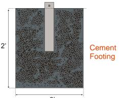
2' \*\*This illustration shows the bolt hole exposed, however some customers elect to mount the sleeve flush with the ground to avoid hitting the sleeve with lawn maintenance equipment.\*\*
