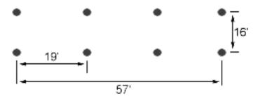
The overall frame is designed to be approximately 57' long by 16' wide, however the corner fittings have some adjustability, so you can compensate for uneven ground. We recommend that you make the frame as large as possible in order to allow the net to slow a ball more before it hits the frame, reducing the speed of ricochets.
