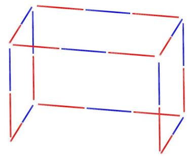
\*\*Make sure to insert the poles all the way into the fittings. The bolts are not for the holes in the poles. They are used to set the poles in the fittings.
