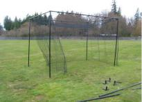
Complete the framework using the remaining poles and fittings As shown. Use the two-way (90°) fittings at the bottom front. Fasten the sides and bottom of the net to the frame using the Remaining hook-and-loop fasteners.
