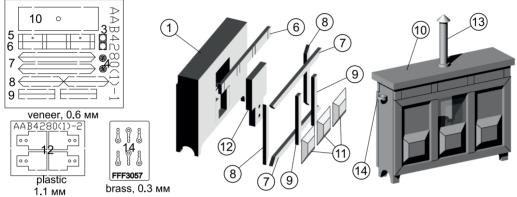
Remove the base of the binnacle from the plate (1) and remove the deposit from it. Make a semi-circular cut in the area of the legs of the binnacle (circled in the picture) with a needle file.
