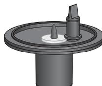
5. Squeeze Duck-Bill Valve to open mouth and free any build-up. Rinse and dry. Ensure part is properly inserted onto Spirit Lid Center before use. Not having Duck-Bill Valve in place will cause Spirits to leak.
