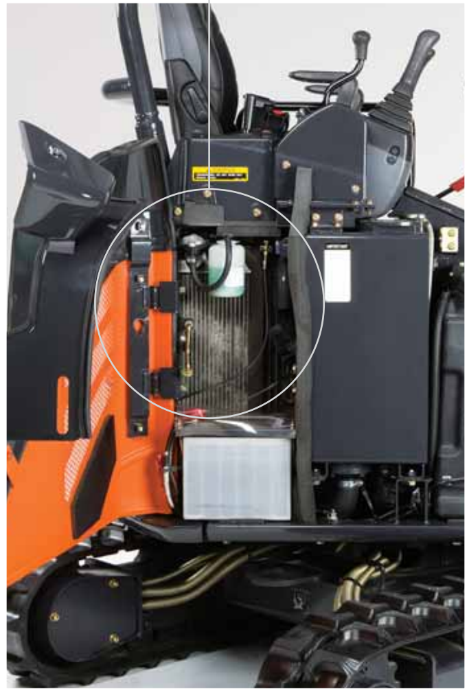
Inspection points are concentrated for quick daily maintenance.
