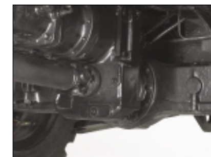
The undercarriage is a welded stress-relieved structure. The drive system has a two-gear power-shift transmission and variable-displacement, axial-piston-type travel motor. The front axle can be locked hydraulically in any position.
