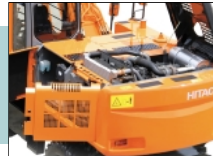
A low-noise muffler and the Isuzu Tier II emissions control engine ensure a quieter, more environmentally friendly excavator.
