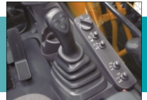
Switches and other essential controls are located near the operator, enhancing control and minimizing fatigue.
