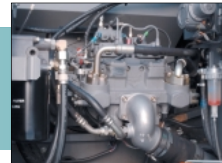
The engine oil filter and water separator are positioned for easy access from the ground.
