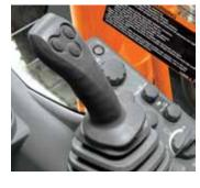
Ergonomically correct short-throw pilot levers provide smooth, precise fingertip control with less movement or effort. Pushbuttons in the right lever allow fingertip control of auxiliary hydraulic flow for operating attachments.
