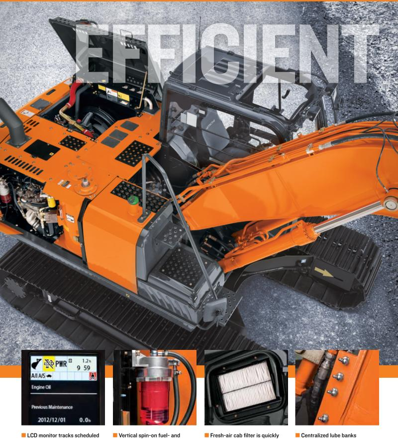
maintenance and reminders. Should a problem arise, it provides diagnostic codes to assist in troubleshooting. ZXLink™ can also provide early warning and remote diagnostics.
