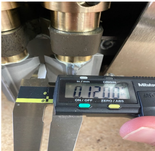
Figure 8 Measuring Cutter Gap
