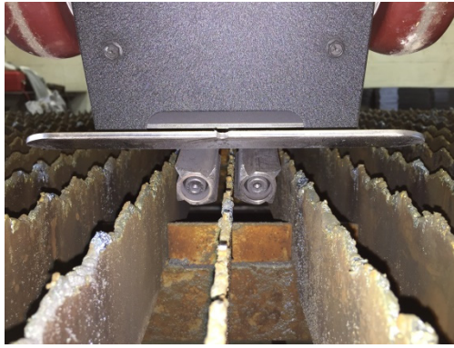
Figure 4 Cutters shown centered on slat
