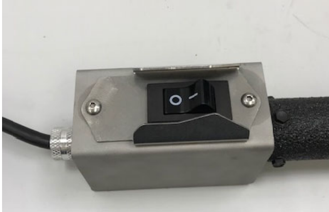
Figure 1 Rocker switch on handle end, in off position, acts as circuit breaker reset in case of over-current
