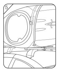
Place the boat on your roof bars with the hull facing the upright
