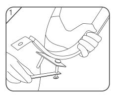
Remove the nut and washer from one side
