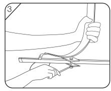
The roof bar thickness must be no more than 28 mm this will ensure the nuts lock securely
