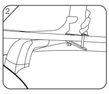
Place the upright onto your roof bars. Tighten both sides equally until secure. Do not over tighten
