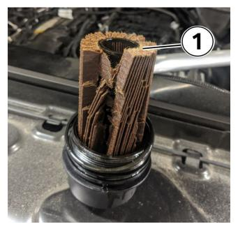
For example, the filter paper is torn, and the lower plastic section remains stuck inside the engine oil filter housing (1).
