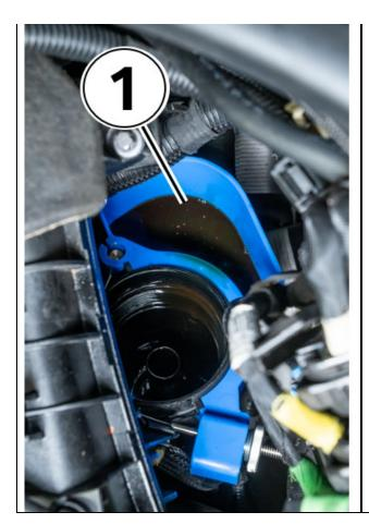
Photo shown with oil filter housing cap and filter removed.
