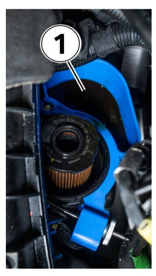
8. Slowly remove the oil filter housing cap and the filter insert.
