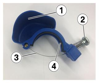
1. Install special tool 83 30 5 A3B 354 BMW Oil Catch onto the side of the oil filter housing.
