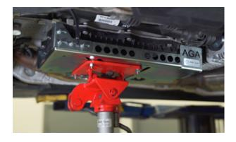
Use – for support of the various versions (including hybrids) of 8HP transmission during removal and replacement.
