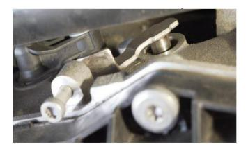
The 8HP Park Release Tool will not work on this style park lever. Please note the adjustment screw.
