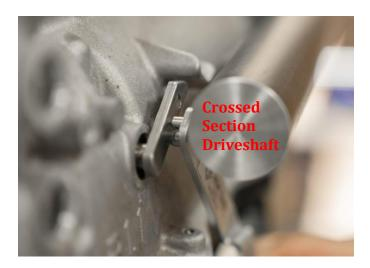
1. On X-Drive vehicles where the driveshaft obstructs your view, use the post on the lever to guide the lever onto the release lever. Do this by pushing the lever up directly above the center transmission pan bolt until it makes contact to the release lever. Slide the lever back and let it drop into the hole.
