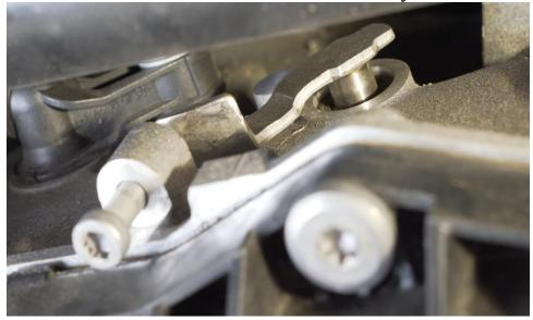
The 8HP Park Release Tool will only work on this style 8HP transmission:
