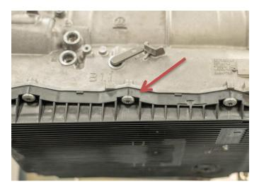
1. To install the 8HP Park Release Tool, locate the center bolt of the transmission pan. The release lever is located directly above the center transmission pan bolt.
