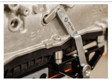
4. Use the center bolt of the transmission pan as a point of reference; bring the lever up and install it into the release lever of the transmission.
