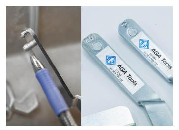
3. Included in the kit are two different types of levers, a short and long lever. Most 2wd vehicles will use the short lever and most X-Drive vehicles will use the long lever. On the backside of the lever, there is a post that helps you guide the lever onto the release lever. This post will be very helpful when working on X-Drive vehicle.
