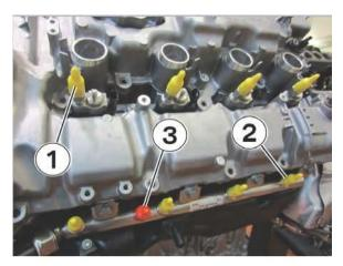
2. Install a yellow cap onto each of the injectors (1) and the high-pressure fuel supply rail (2).
