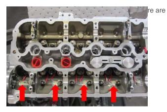
e 11. Block all four holes with a standard white lithium grease. See arrows.
