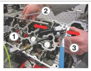
39. Remove the compression lever rod (1) from the compression plates (2) located on the camshaft bearing caps.
