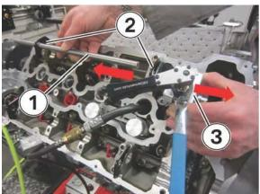
25. Remove the compression lever rod (1) from the compression plates (2), located on the camshaft bearing caps.
