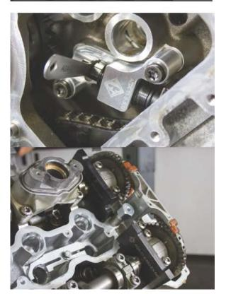
46. Cam Timing is correct when timing chain is in correct tension with AGA chain tensioner tool (AGA 11-9-900), or BMW equivalent, and cam plates (AGA-11-9893-IN-N63) & (AGA-11-9-893-EX-N63) rests without gap on the cylinder head.
