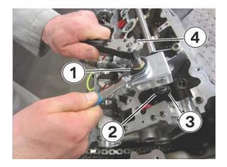
32. Rotate the compression nut (1) counter clockwise until the compression foot (2) depresses the valve spring (3).
