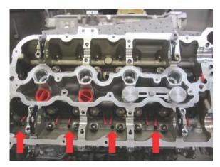
8. Install the eight supplied plug brushes (1) into the eight oil drain back holes (see arrows) in the cylinder head, located on either side of the head bolts.
