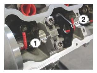
13. Exhaust camshaft position: Reinstall the "LA5" exhaust camshaft bearing cap (1) with a compression plate (2) onto the rear of the cylinder head.
