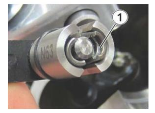
35. Apply a small amount of white lithium grease to the keeper grooves (1).
