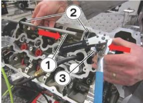
30. Install the valve spring retainer (1) and valve spring (2).
