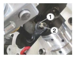
33. When the valve stem is exposed (1), apply a small amount of white lithium grease (2) with a brush to assist in holding the keepers in place.
