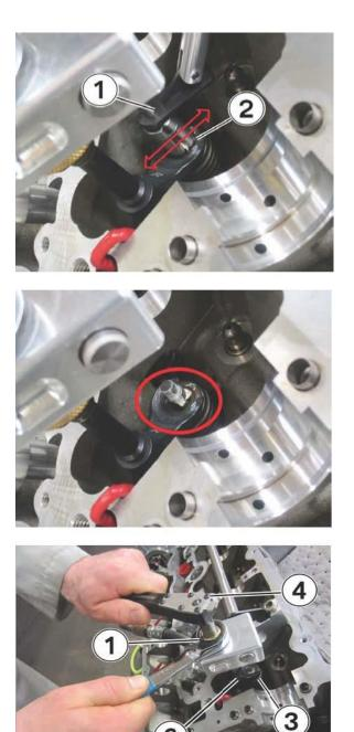
36. Place the N63 keeper tool with keepers (1) over the valve stem (2), and move the tool gently side to side to release the keepers (see arrow).
