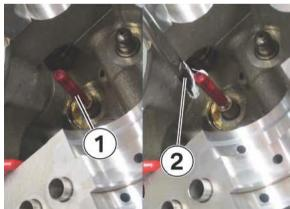
27. Remove the valve seal (1) with the seal pliers (2) included in the kit. Part #: AGA-SRP-N63
