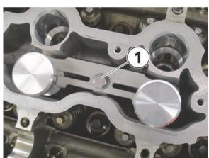
7. Install the two red plugs into the remaining open injector bores (1), so that debris does not fall into the cylinders while performing the repairs. Part #: AGA-IBPP-N63
