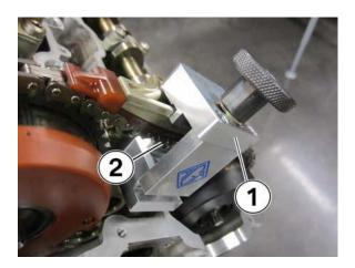
18. Install the timing chain holder (1) onto the opposite cylinder bank timing chain guide rail.
