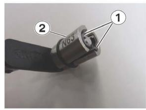
34. Install the keepers (1) into the N63 valve keeper tool (2) supplied in the kit. Part #: AGA-N63-6mm-VKT
