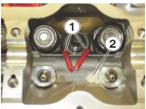
12. Exhaust camshaft position: Using two of the four bolts that hold the high-pressure pump housing, install the cam bracket (1) and a compression plate (2) onto the front of the cylinder head, above the cylinder 1 ignition coil bore.
