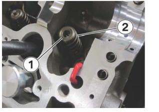
26. Remove the valve retainer (1) and valve spring (2) to expose the valve seal.
