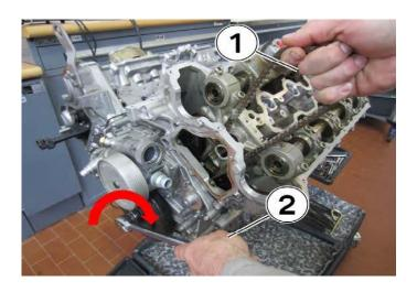
49. When cylinder bank 2 valve seal replacement is complete, the crankshaft has to be positioned 150° before cylinder 1 TDC.
