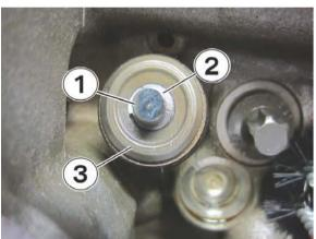
40. Wipe away excess grease. Inspect the valve stem (1), keepers (2), and the spring retainer (3) for the proper alignment before continuing.
