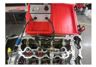
19. Use a cylinder leak-down tester to supply air pressure to the cylinder. The air pressure will hold the valve in the closed position while removing the valve spring retainer, valve spring, and keepers.
