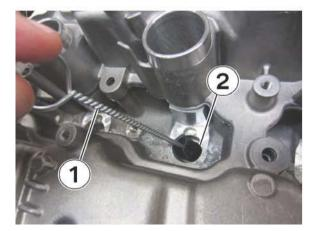
4. Gently clean the upper portion of the injector bores with the brush before installing the fuel injector-sealing plug. Part #: AGA-HB-8-34
