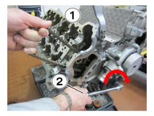
43. When cylinder bank 1 valve seal replacement is complete, the crankshaft has to be positioned 150° before cylinder 1 TDC. Hold the timing chain with one hand (1) and rotate the engine (2) in the direction of the arrow. Do not allow the timing chain to get jammed. Do not forget to remove the brushes from the oil return holes. Clear the oil return holes covered with grease, using a small brush or cotton swab
