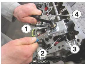
21. Slide the compression lever rod (1) into the compression plates (2) located on the camshaft bearing caps.
