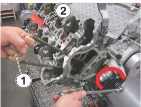
16. Screw four of the black plastic spark plug TDC tools (1) into each of the spark plug holes (see arrows) to avoid debris from falling into the cylinders.
