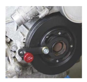
50. When the crankshaft is positioned correctly, install AGA-11-8-570 Crank Holder and AGA-11-9-190 Pin, or BMW equivalent tools.
