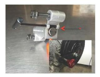
Pin will keep piston in retracted position for tensioner removal. Rotate engine clockwise slightly to push timing pin back in front cover timing groove
