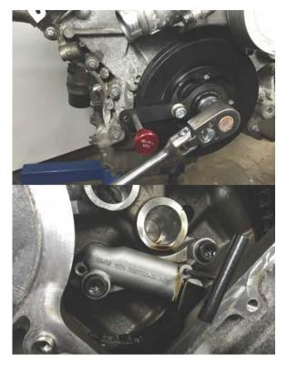
7. Pull back timing pin. Turn engine very slightly counter clockwise to collapse hydraulic chain tensioners enough to push in locking pin. See picture.
