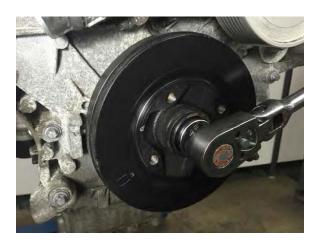
1. Turn engine over with 27mm socket in clockwise direction until mark on balancer is close to timing groove in front cover.
