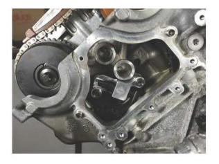
13. Transfer bolts from stock chain tensioner to chain tensioning tool (AGA-11-9-900). Tighten T40 bolts to 13nm.
