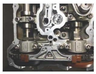
Note: when in correct position small flat on cams is facing up on intake and exhaust cams both banks
