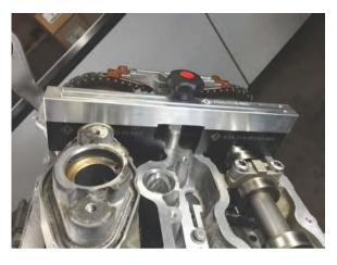
5. Install 12mm to 8mm adapter and hold down bar AGA-11-9-892 tighten firmly by hand
