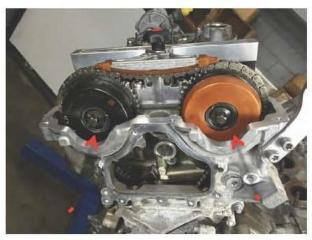
Loosen E14 M10X1 cam adjuster bolts. Remove cam plate, hold down intake and exhaust plate. Remove 12mm to 8mm adapter.
