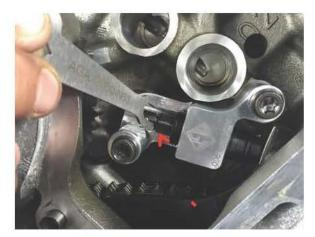
14. Tighten adjuster by hand to remove chain slag. Tighten with 10mm open end wrench until gauge tool (AGA-G060-N63) can just be inserted between 10mm hex and round end. Lube with copper anti-seize under bolt head.
