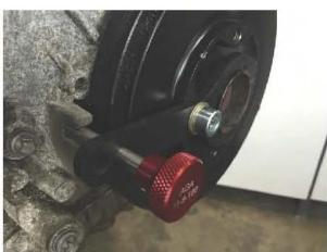
Install AGA-11-8-570 facing balancer. Turn engine over slowly in a clockwise direction until pin just drops in timing groove. This sets the engine to 150° before cylinder number 1 firing TDC.
