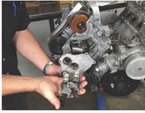
6. Remove cam solenoids and timing cover, exposing timing chain tensioners.
