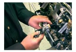
**11. Valve Stem Seal Removal:** Remove the valve spring and retainer and if you have a pair of "fuel hose type pliers" it makes it much easier to remove the valve stem seal.
