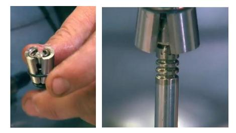
15. Now switch the rotation of the lever on the ratcheting wrench and release the tension on the spring. Watch the keepers while doing this to insure that they don't get pushed off accidentally. Release the compressed air in the cylinder.
