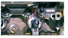
Install the brush plugs in oil return holes on the bank you are working on, R side (Bank 1) has 4 holes and L side (Bank 2) has 5 holes. The brush plugs are VERY IMPORTANT in case you accidentally drop a keeper the brush plugs will prevent it from falling down into the oil pan.
