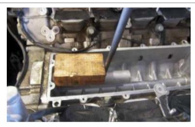
4. Pull tube out with lever bar.
