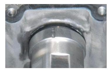
9. Rotate rear ring so the machine notch is straight up. Angled side is towards rear of engine block and o-ring. Tighten tube by hand until it has tension on front and on the rear o-ring.
