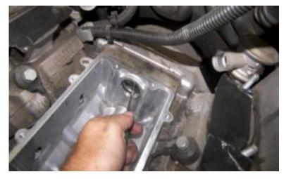
6. Remove rear o-ring in back of engine block.
