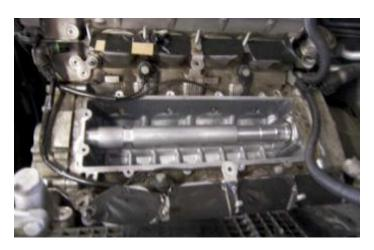
8. Start with the tube collapsed. Lube tube on both ends with white grease (supplied in kit). Hold tube into engine block. Insert tube into rear of engine block. Turn tube so it expands, as front of the tube enters seal; observe front seal with mirror from water pump side as the tube goes into seal. Seal cannot be pinched. If seal pushes out, collapse tube a bit, turn tube without expanding a few turns and then continue expanding until seal can no longer be seen from water pump side.
