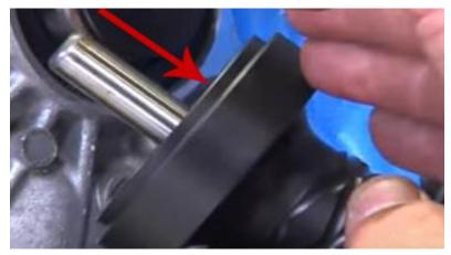
NOTE: The seal installer has a machine step that ensures the seal is installed to the correct depth. The seal installer works on the right and left side of the transmission. Please remember to have the centering mandrel installed when using the tool.
