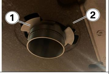
The universal oil drain splash shield (1) is installed in a vehicle with a plastic under body cover (2).
