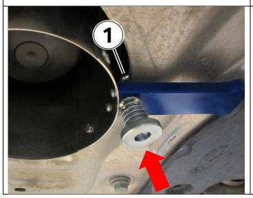
For hands free operation the hook portion of the tool needs to be pushed upward in the direction of the arrow and then rotated (1) to secure the tool in place.
