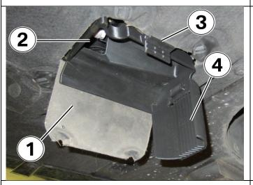
Open the engine oil drain plug access port (1).
