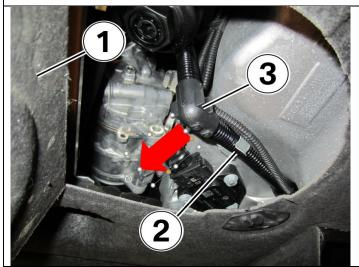
Open the engine oil filter access port (1).
