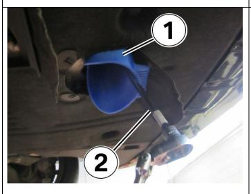
Install the oil filter splash tool (1) onto the oil filter housing. This will take some effort to position it correctly around the oil filter housing. The tab on the front of the tool needs to point forward and it will also hold open the access port.
