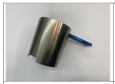
Special tool P/N 83 30 5 A7B 9C9 – N63 Oil filter Splash Shield tool for N63, N63TU, S63 and S63TU.
