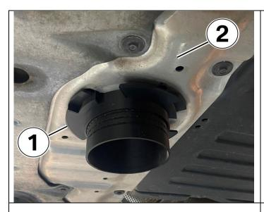
The universal oil drain splash shield (1) is installed in a vehicle with a metallic stiffening plate (2).
