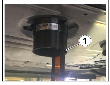
The engine oil drain plug has been removed - the oil is directed straight downward (1).
