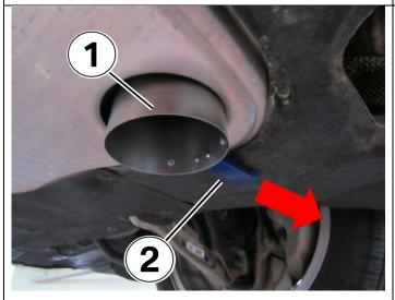
Install the splash shield (1) around the oil filter with the handle (2) in the direction of the arrow pointing directly towards passenger rocker panel.
