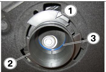
After the tool is installed (1) rotate the threaded center portion (2) of the tool clockwise until the seal contacts the engine oil pan (3).
