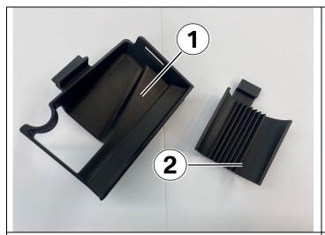
Special tool P/N 83 30 5 A7B 9D4 - B3X-B4X Oil Drain Splash Shield.
