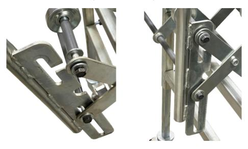
Figure 2 - Engaging the Handle/Package Stop into the Raised Position
