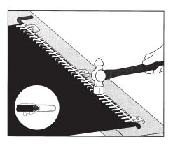
**6.** Hammer lacing completely into top of belt.
