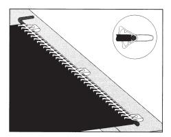
**3.** With bar side up, center lacing on belt holding belt against guage pin.
