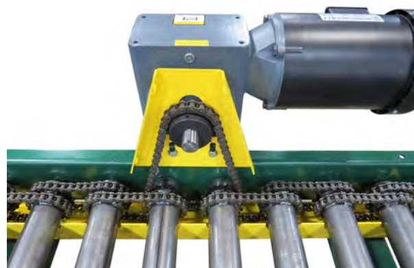
Drive with Guards Removed
