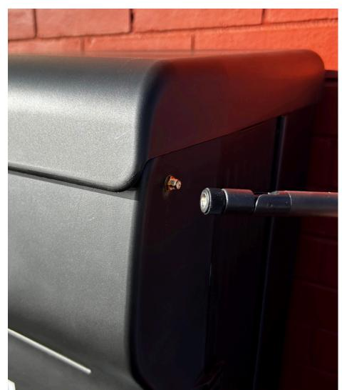
8. Screw the antenna clockwise until it is fitted correctly. Turn the antenna so that it is pointing upwards.
