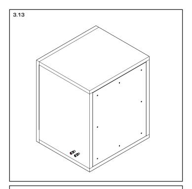
· Use the supplied black wood screws to screw the back door in place. Use enough torque to compress the gasket tape, but not enough to pull the screws through the countersunk holes.
