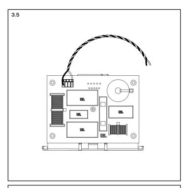
· Insert one end of the internal input wire into the crossover where it says IN+ and IN-. Use the orange wire for (+) and the black wire for (-). Tighten the corresponding screw posts with the small flathead screwdriver to hold the wires in place.
