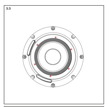
· Carefully flip the coaxial unit over and place it magnet side down. You will need to support it with one hand while you unscrew the 3 screws holding the crossover bracket onto the lip of the speaker.
